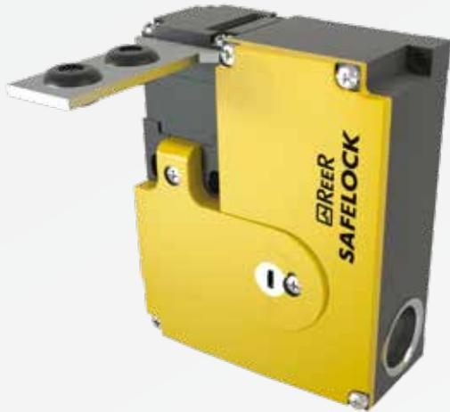
Safelock is a safety switch utilised in the protection of personnel when opening doors leading to dangerous areas. It acts by monitoring and interrupting the safety circuit during dangerous scenarios.
