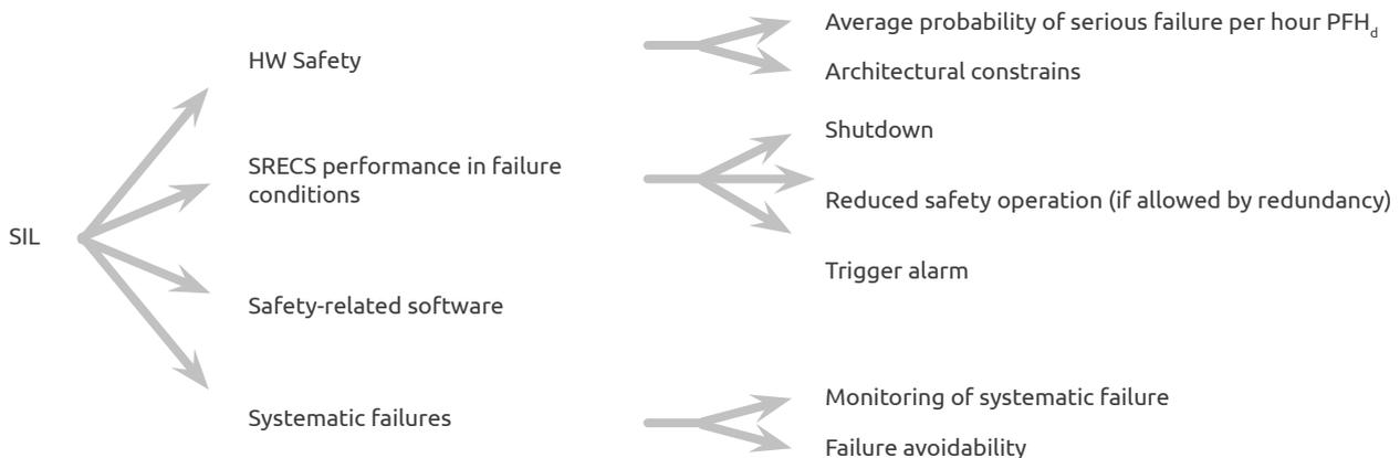
Each subsystem shall consist of electrical circuits suited to attain the required SIL.
