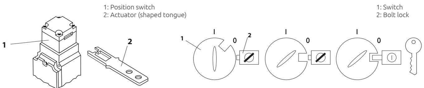
Fig. 9. Type 2 interlocking device - Coded
