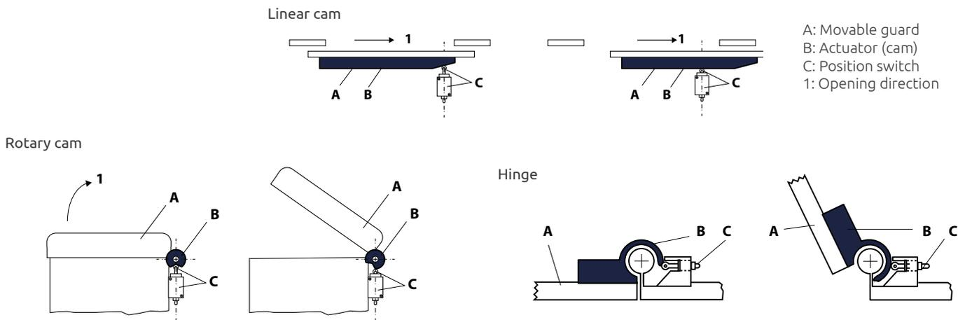
Fig. 8. Type1 interlocking device
