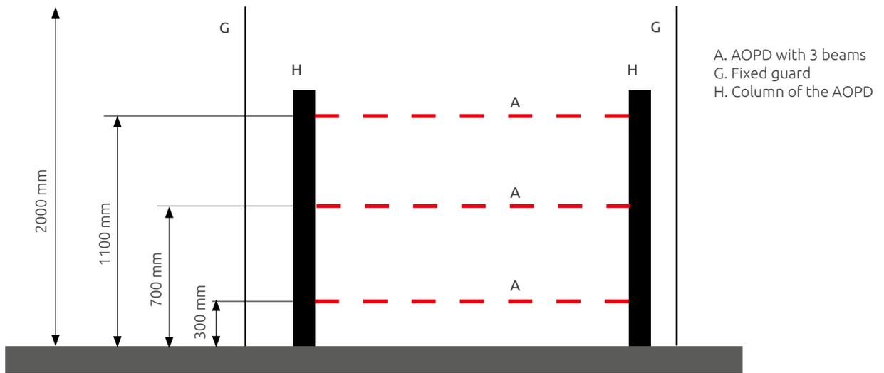
Fig. 23. Positioning of the AOPD - General
