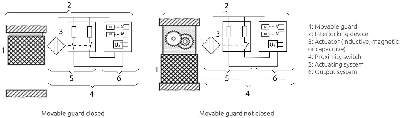
Fig. 10. Type 3 interlocking device with proximity switch actuated by uncoded actuator
