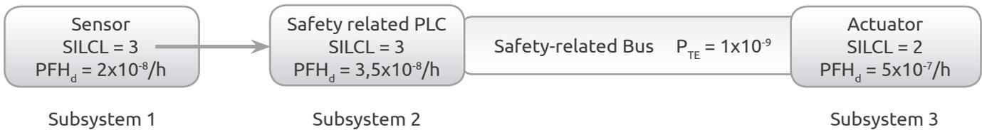
$$PFH_d(\text{system}) = PFH_d(ss1) + PFH_d(ss2) + PFH_d(ss3) + P_{TE} = 5,56 \times 10^{-7}/h$$
