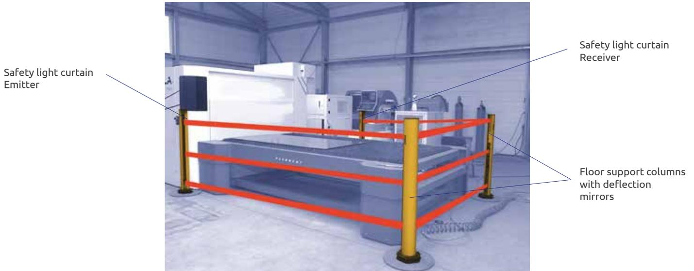
Fig. 26. Machine for laser cutting perimeter protection
