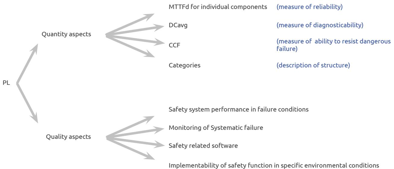
Fig. 3. Mandatory qualitative and quantitative requirements to be met for safe control system design to ISO 13849-1
