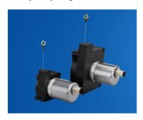
To measure linear movements or linear displacements, an absolute magnetic rotary encoder can be combined with a draw wire sensor. The contact-free measuring sensor stage of the MCD Sensor doesn't have any abrasion. The sensor can directly be connected to digital control units via SSI- or CANopen or Analog Interface.
