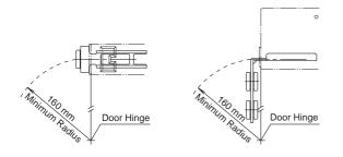
When the door hinged is on the extension line of the actuator mounting surface:
