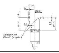
• Using the HS9Z-A65/A66 Angle Adjustable Actuator
