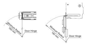
When the door hinge is on the extension line of the interlock switch surface:
