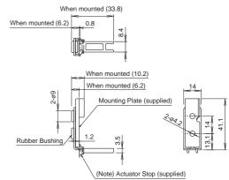
Note: The actuator stop is used to adjust the actuator position. Remove the actuator stop after the actuator position is mounted.
