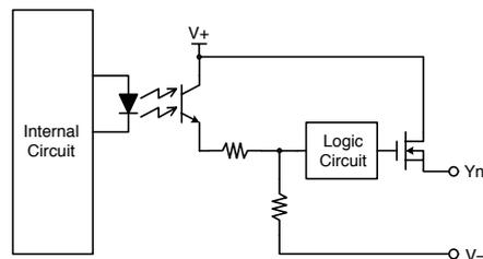
The operating characteristics of the monitor output change depending on the selected logic. For details, see user's manual "Chapter 5 Logic." The basic specifications remain the same.
