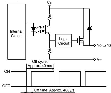
The safety outputs of the SafetyOne are solid state outputs. When the output is on, off-check signals are generated at regular intervals. The operating characteristics of the safety output change depending on the selected logic. For details, see user's manual "Chapter 5 Logic." The basic specifications remain the same.
