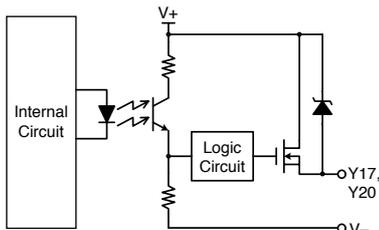
The selected operating characteristics of solenoid/lamp output change depending on the selected logic. For details, see user's manual "Chapter 5 Logic." The basic specifications remain the same. Do not use solenoid/lamp output as a safety output, otherwise the system's safety cannot be assured when the SafetyOne or safety components fail.
