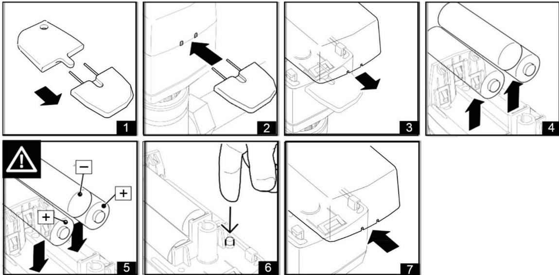
**NOTE** - Insert the batteries with the correct polarity marked in the battery compartment. Only use alkaline batteries (type: AA, LR6 1,5 V). Do not use rechargeable batteries.
