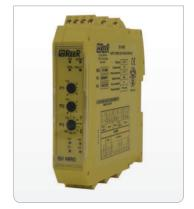
P1 and P2 selectors allow to set numeric values from 01 to 99. P2 selector allows to set a multiplier to apply to the numeric value obtained with the first two. The multiplier can be set in "Hz" or in "rpm" (round per minute). Note: Only when the proximities switches sensor show a single pulse per turn, the value in "rpm" corresponds to the value in "ipm" (pulse per minute).
