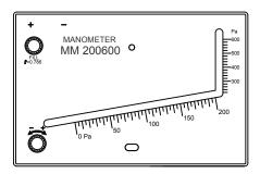
4) Connect the pressure tubes. Connect positive pressure to port labeled "+" and negative pressure to port "-".
